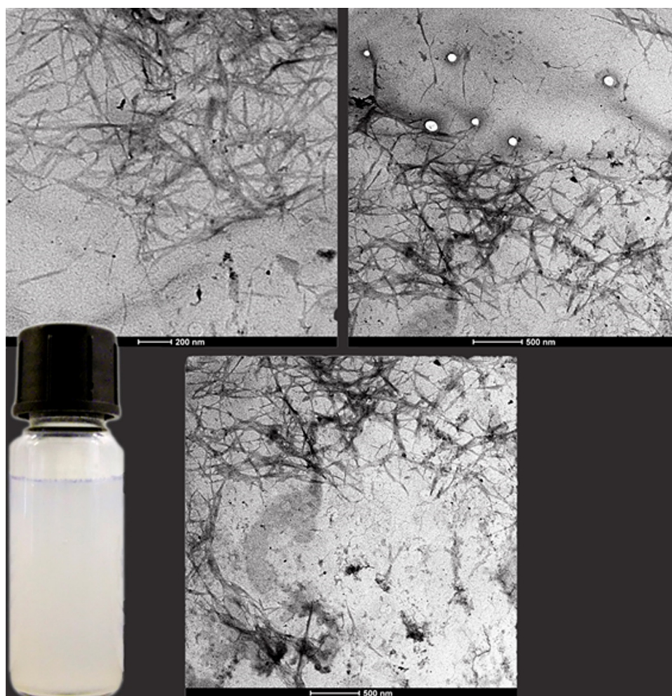
Fig. 5. TEM pictures for cellulose nanocrystals from the bleached acetosolv pulp (BAP), and a picture of a sample of the nanocrystal suspension.
